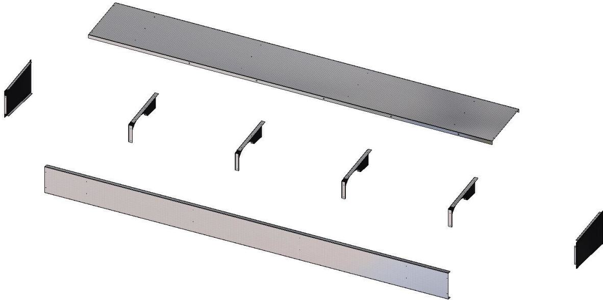
Exploded Assembly View for One Piece Hood
